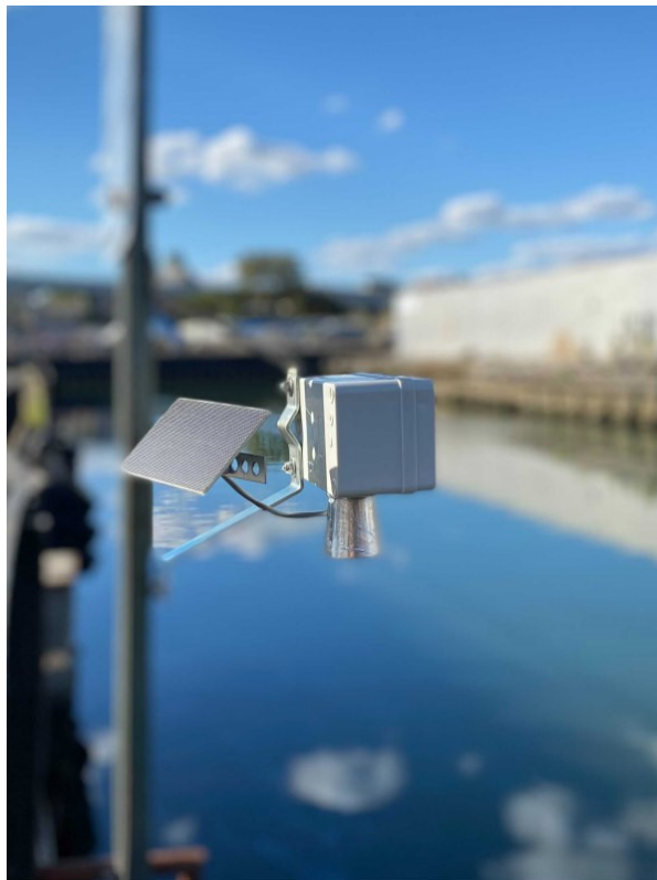
One of the initial sensors deployed is over the Gowanus Canal to monitor water level changes due to tidal influence.
